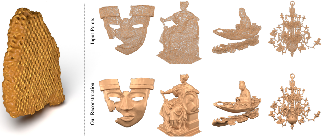
Fig. 1. The reconstruction of a 3D scan of a beehive (left) and comparisons of input points and our respective reconstructions on the Objaverse dataset (right) [1]. These examples show the capability of our neural distance field encoder to capture a large amount of detail in a single forward pass, using only oriented point clouds as input.
