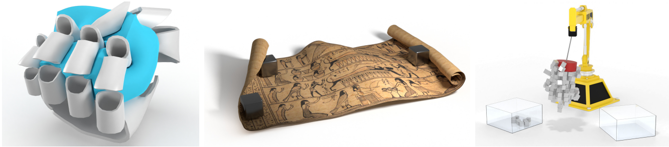
Figure 4: A selection of energy-based multiphysics simulations with strong coupling. Left: A robotic hand modeled by rigid bodies, joints and motors compresses an elastic cube [FLL*24]. Middle: A scroll modeled as a Cosserat shell is pushed open by rigid bodies through frictional contact [LFFJB24]. Right: A crane modeled as a multibody system lifts metallic cubes using magnetic forces that are strongly coupled with frictional contact [WFFJB24].
