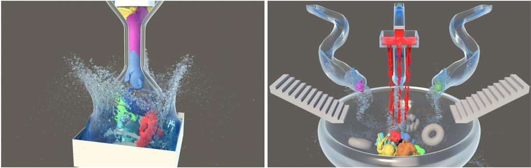
Fig. 1. Left: Stable simulation of eight walrus models (210k particles) that are pushed through a tight funnel and impact the water in a container with 1.2M fluid particles. Right: To showcase the coupling capabilities of our method 10 deformable solids and 4 rigid tori are dropped into a bowl while water and a highly viscous fluid are poured on top. A total of 800k particles are used for the fluids and 252k for the elastic objects.
