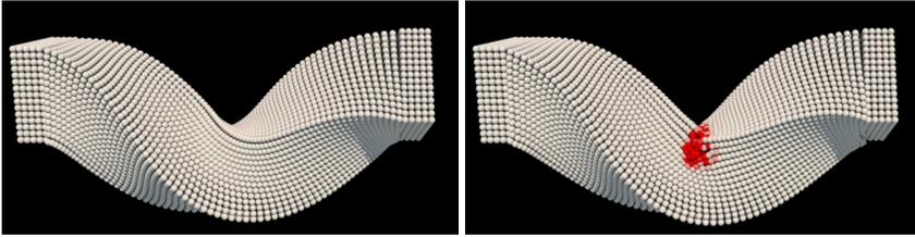
Fig. 4. Twisted beam experiment. Our implicit zero-energy mode correction successfully produces a stable simulation (left) while the explicit handling proposed by Ganzenmüller does not (right). Particles colored in red experience very high velocity.
