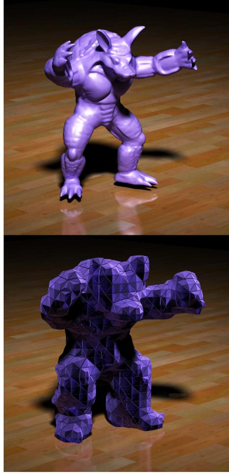
Figure 1: The Armadillo (top) converted into a tetrahedral mesh (bottom).
