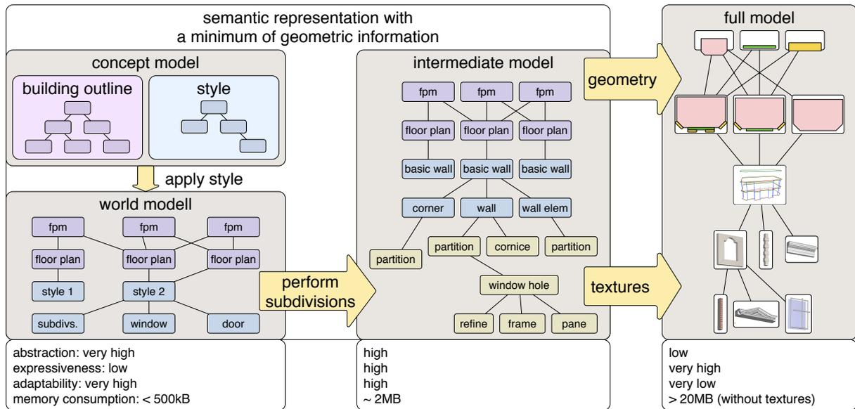
**Figure 3: Modeling work flow. From the abstract concept model to the geometry (full model).**
